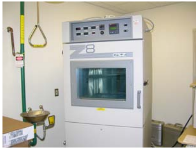
Figure 3: Image of Thermal Chamber. The boards slide in sideways And air blows at the boards from the back.
